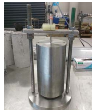
Figure 5. Apparatus used to measure the coefficient of thermal expansion.
