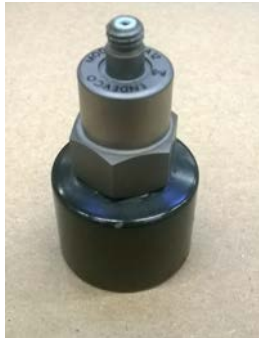
Figure 11. ENDEVCO 752A12 accelerometer with a magnet base.
