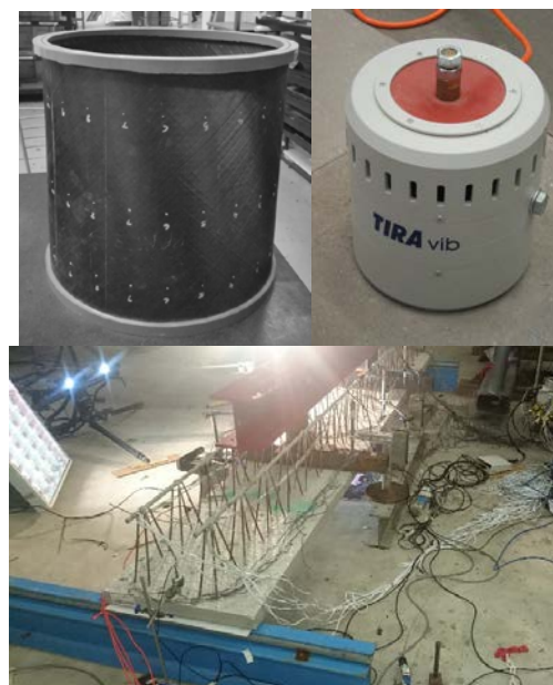
Figure 1. Some of the tested objects: a carbon fibre cylinder (top right), shaker (top left) and concrete slab/planck (bottom)
